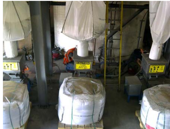
Figure 6: Supersac Loading System
