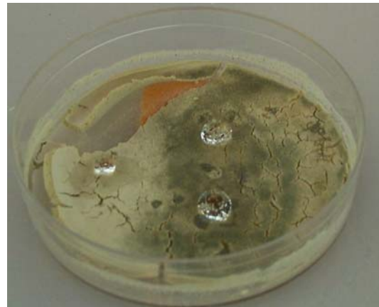
FIG. 11 HYDROPHOBICITY OF APATITE SURFACE TREATED WITH MO WITH BACILLUS POLYMYXA AS ESTABLISHED BY FROTH FLOTATION
