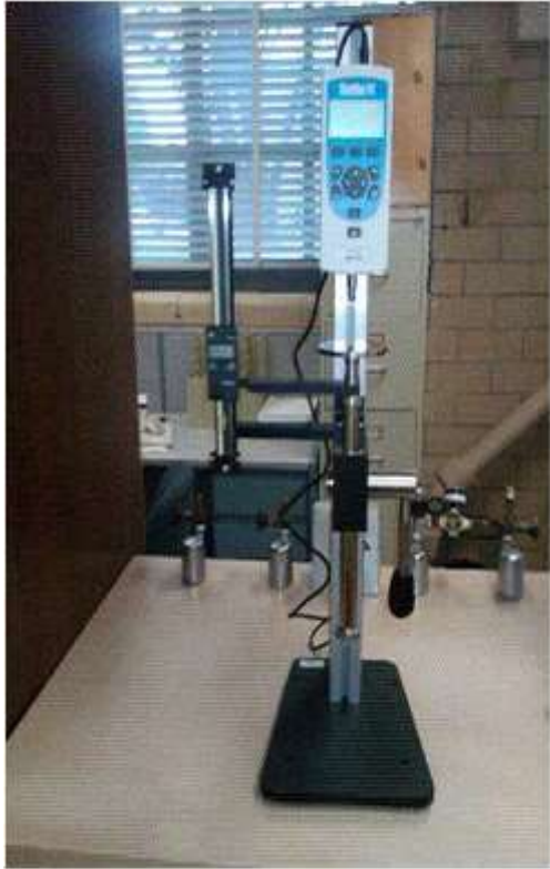
Figure 4. Digital Break Force Gauge with Mechanical Test Stand
